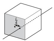
When viewing the shaded face, what is the torque of the couple that will now be needed to stop the cube from toppling?
